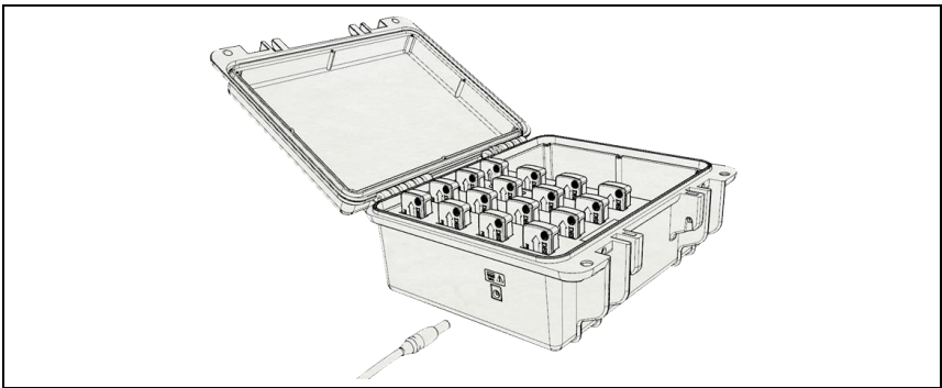
Figure 3: Trigno System “Charge-16” Station for sensor recharging. No wireless or digital communication is available on the Charge-16 component of the system.
